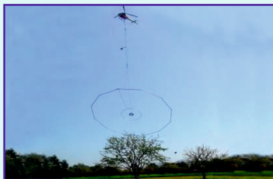
Fig.3 : Heliborne geophysical survey by AMD
